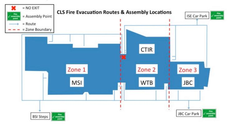
Activation of the fire alarm (continuous alarm) in one building causes the immediately adjacent building(s) to go into alert (pulsed alarm), thus:
